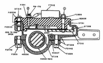
yet be free to move when the spark is advanced or retarded. This fit is controlled by the clamping action of the lower screws in the sketch and the thin gasket between the upper and lower halves of the casting.
